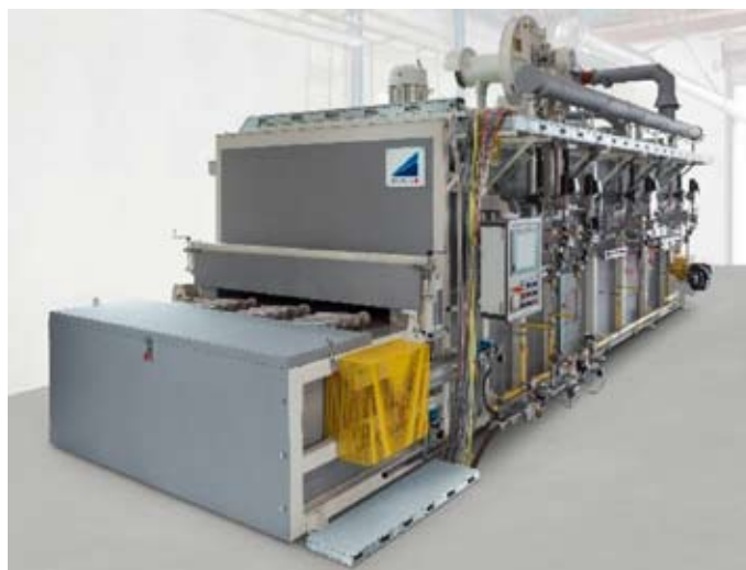
Heat treatment system for automotive suspension components
