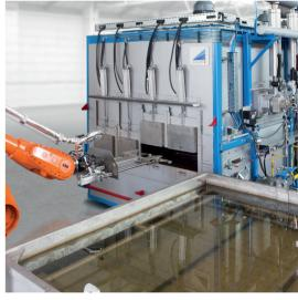
Exit end of solution heat treatment furnace for aluminum with robot and quenching tank
