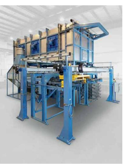
Apart from continuous conveyor furnaces, we also offer indexing pusher furnaces for artificial aging of forgings. These systems likewise provide fast and uniform heating, a quick return of parts into the processing workflow and, above all, substantially reduced space requirements.
