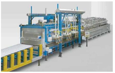
schwartz chamber furnaces serve to heat aluminum products of any geometry, from bulk parts in transport containers through ingots or billets to aluminum components arranged on trays.
