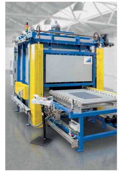
For semi-hot and hot forming of aluminum sheets, we offer you our patented application with high convection Jet Heating that has been successfully tested in our in-house Technology Center many times.
