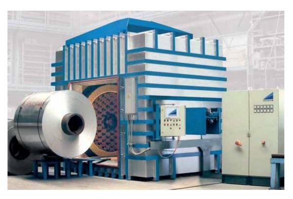
Jet rotation heating combines jet heating with a rotation of the nozzle banks. This patented system has been developed by us specifically for perfectly uniform heating of aluminum strip coils.
