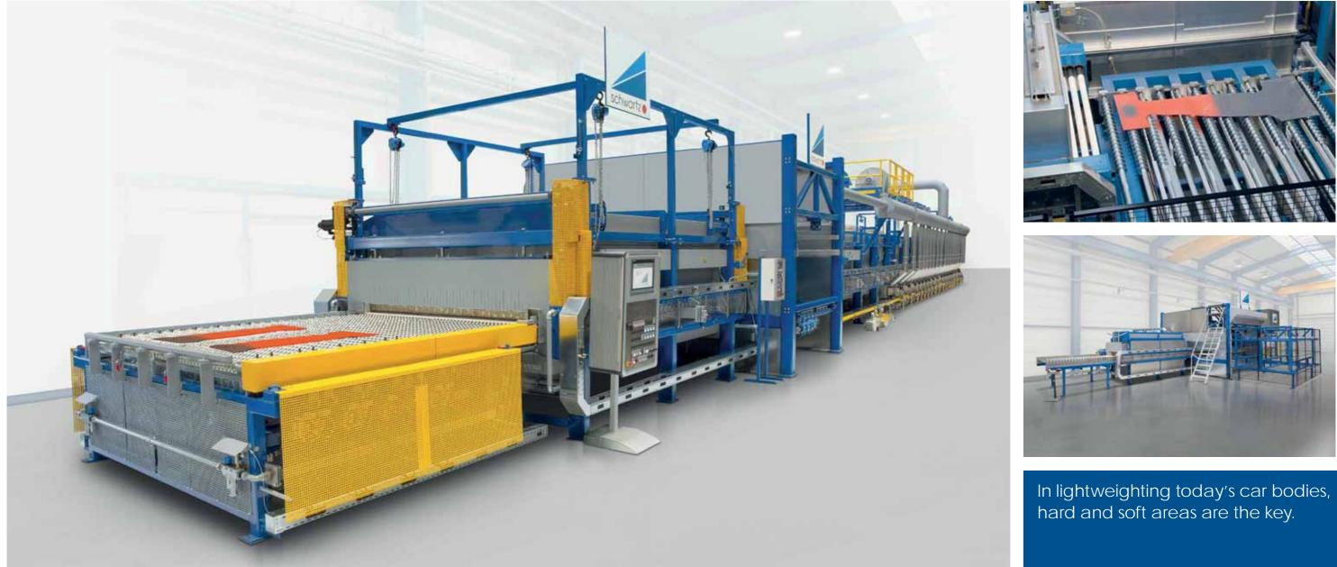
The thermal printing technology, first launched and established on the market by our company, allows two or more different temperature zones to be realized in the same blank. The distinct regions are subjected to a selectively focused heat treatment, i.e. application of locally modified time-temperature curves.
