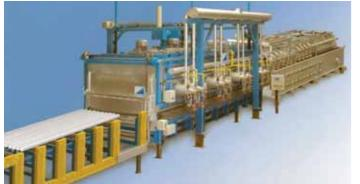
Since our company's foundation in 1984, we have built and commissioned more than 200 heat treatment systems for aluminum, custom-designed to satisfy individual requirements. All these systems feature adjusted highly efficient atmosphere recirculation technology as well as product-specific nozzle systems to ensure fast, effective and uniform heating.
