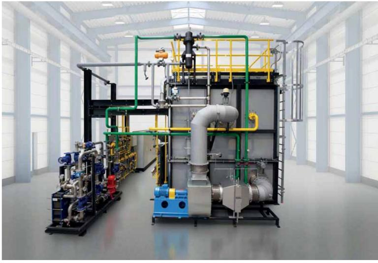
In this furnace, coils of copper and copper alloy strip can be heated and cooled quickly and uniformly without causing mechanical damage to any part of the surface. The maximum temperature difference reached is 10K.
